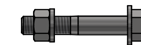
VIEW14 3/8"-16UNC x 2 1/4" HEX CAP SCREW, FLAT WASHER, LOCK WASHER, HEX NUT
